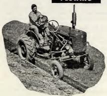
Farmall Touch-Contral an this Farmall Super-A tractor lawers and raises the plaw bottom and separately adjusts the drawbar height to change the depth of plawing.
